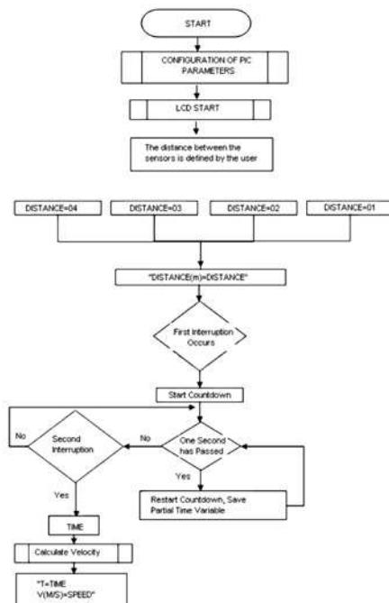
**Fig. 3.** Flow diagram for the microcontroller program. Indicating the sub programs [10].
