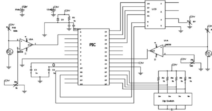
**Fig. 2.** Complete circuit. Description of the hardware used, showing the sensors, operational Amplifiers, electronic devices and their operating configuration, the interface between the PIC and the LCD and the input voltages required for the adequate functioning of the system.
