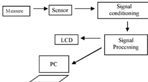
**Fig. 1.** Block diagram illustrating the basic design of the project. The sensor determines the time when the light beam is interrupted, then the elapsed time is defined to calculate the velocity by signal processing (PIC) the LCD is used to show the results.
